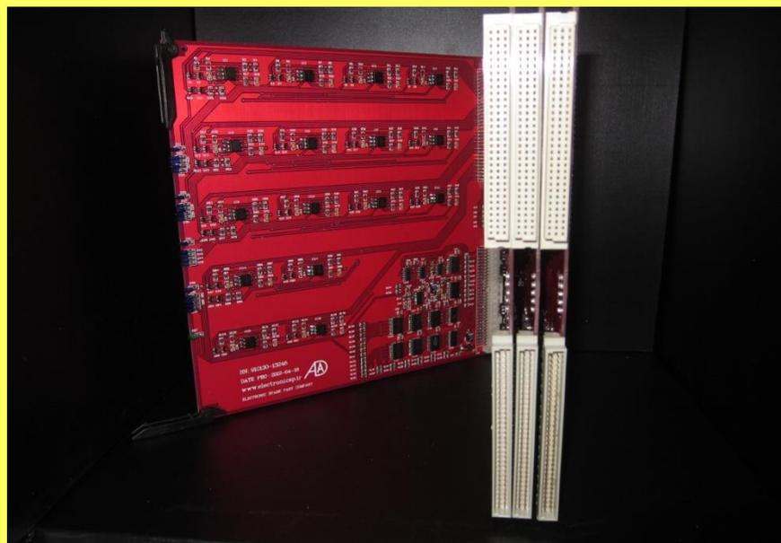
The circuit modules each plug into two electrical connections at the chassis, the lower row of connectors from an industrial standard G64 bus, the upper connects provides input-output connections.
