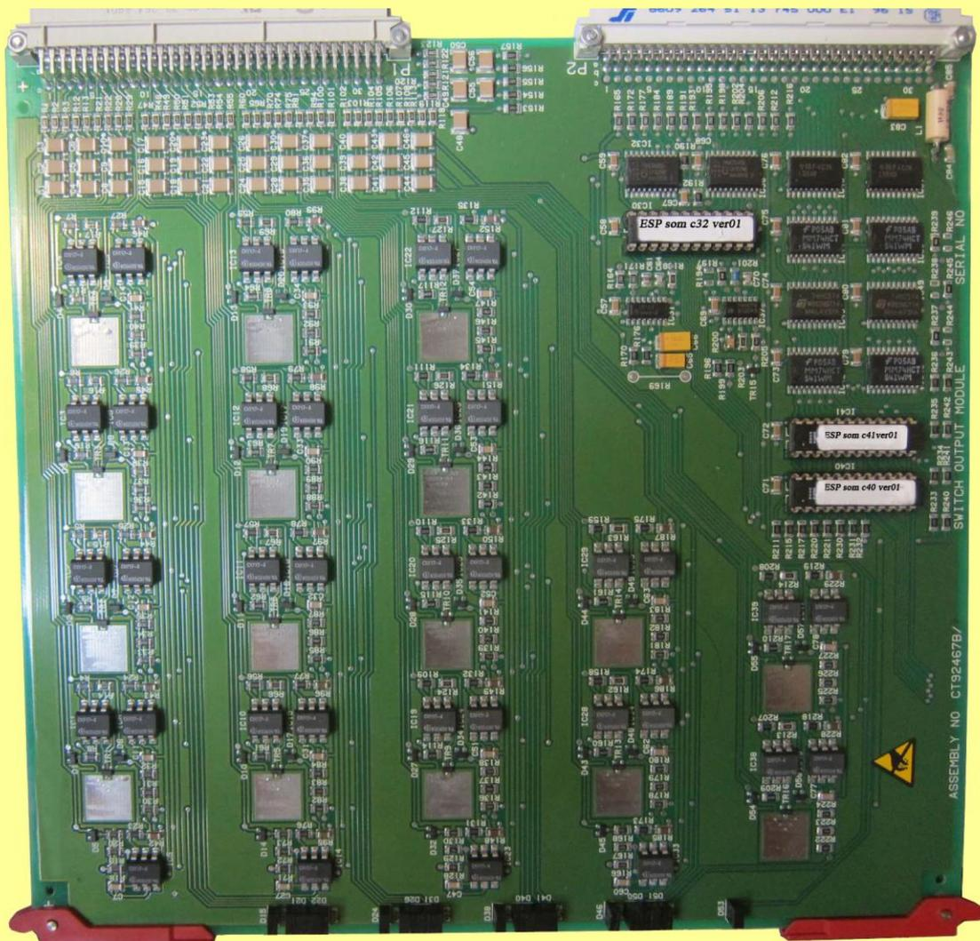
The circuit modules each plug into two electrical connections at the chassis, the lower row of connectors from an industrial standard G64 bus, the upper connects provides input-output connections.
